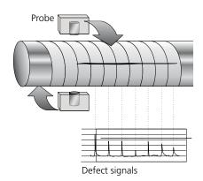
The rotating system scans the test piece in a helical pattern. Every time a probe crosses a crack, it generates a defect signal. In doing so, the rotating system produces a great number of consecutive signals that identify the flaw as a crack. The defect signals appear on the screen as they occur. An angular display shows the position of the defect on the circumference of the test piece.
