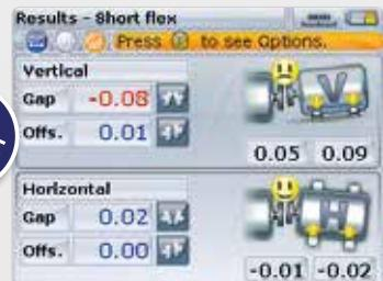
All alignment results are shown in one screen. A smiley and LED clearly display the alignment status evaluation.
